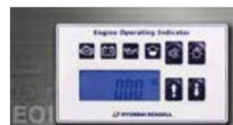
with an additional digital data panel. The EOI and the additional panel can be configured to give the skipper a plethora of information: Engine RPM, Temperature, Throttle Position, Fuel Consumption, Engine Warning and Error Codes and more. The icing on the cake is that Hyundai SeasAll provide an Smart Phone Application, SeasLink. SeasLink makes driving smarter, safer and more fun. Enjoy SeasLink! And also NMEA 2000 adapter provides full-
